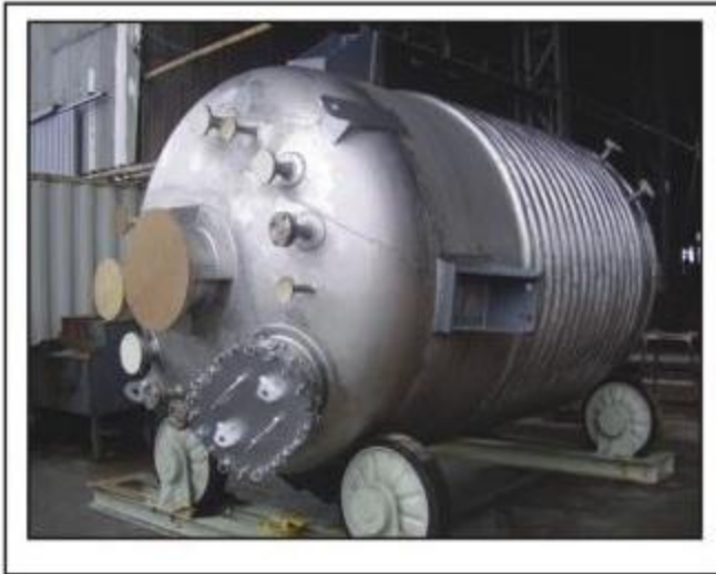
Steam Jacketed Vessel Capacity 10,000 Ltr
