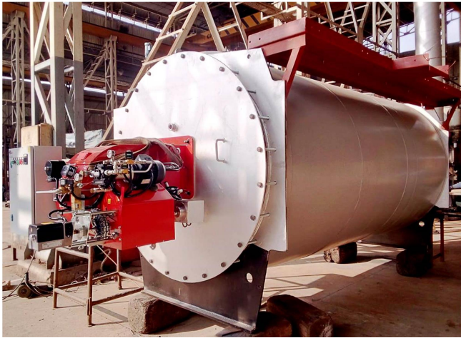
FIRED HOT WATER GENERATOR 2,200 KW CAPCITY for Shaukat Khanum Karachi
