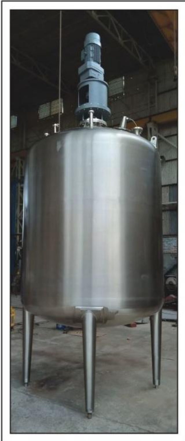
Steam Jacketed Vessel Capacity 10,000 Ltr
