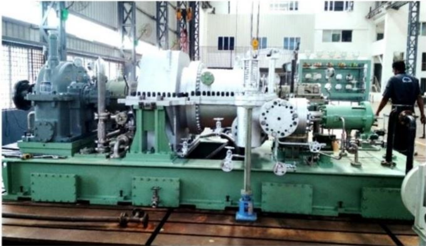
1.6 Megawatt Steam Turbine (MAN)
